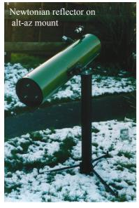
The alt-az is an ideal beginner's mount and is very simple to use. You literally place it where you want to observe from, put the telescope on it, put an eyepiece in the telescope and start observing. It comes in several varieties. It could be a pillar mount where the altitude mechanism is fixed to one side of the telescope, or a tripod where the telescope is usually held in a fork. Or it could be a Dobsonian, known as the Dob. This was developed by the American John Dobson as a very simple
